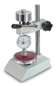
This test stand TI is specially designed for Shore hardness testers and can be purchased optionally together with the HB.
