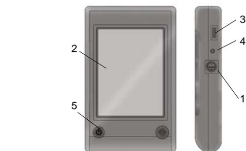
1. Sensor jack 2. LCD screen 3. Mini USB jack
