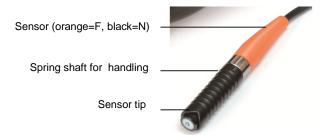
The sensor has to be touched at the lower shaft (pole) segment and it has to be pressed slightly onto the test object.
