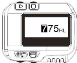
4. By pressing the button
