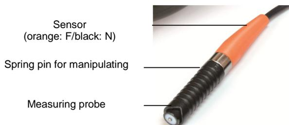
The sensor should be held by the lower pin segment and pressed against the measured object slightly.
