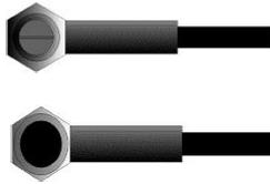
The upper figure is a bottom view of a typical transducer. The two semicircles are visibly separated in the middle of the surface. One of the semicircles is conducting the echoed sound back into the transducer. When the transducer is placed against the material being measured, this is the area directly beneath the centre of the measured surface.
