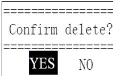
Press the ◀ or ▶ key to move the cursor to 【YES】. Then press the 【ENTER】 key to confirm the deletion of the latest single measured value.
