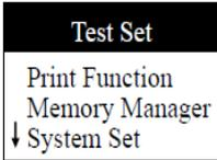
Press **【ENTER】** key to enter **【TEST Set】** menu. Press **【▲】** **【▼】** key to move cursor to the item which will be set, then press **【ENTER】** key.
