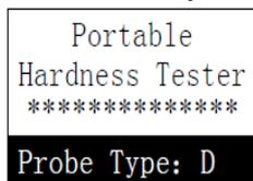
Tester will check and display the type of impact device. At this point carefully observe whether the type is right or not, then enter the main measuring display interface.
