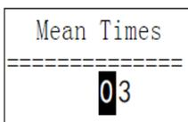
The mean times can be modified in the range of 1~32.
